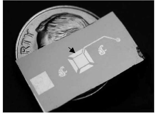
Fig. 8. Photograph of thin-film PZT membrane generator. Arrow denotes one of the four high strain regions.
